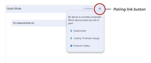
When an instrument is connected, the **button** will turn green. The App is now ready to accept readings from the connected device.
