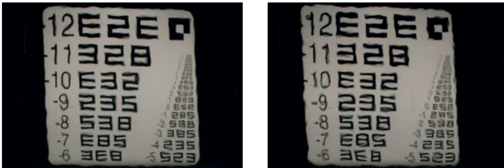
Two highly reflective panels with the same gloss values show little change in DOI but appear different.
